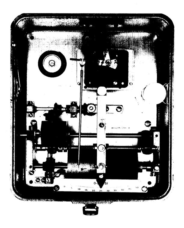
Approval Notice G-56-1, October 16, 1973 covering the Mercor III PT Volume Correcting Integrator describes the operation of the pressure element of that device and the essential description of the Mercor III P.
