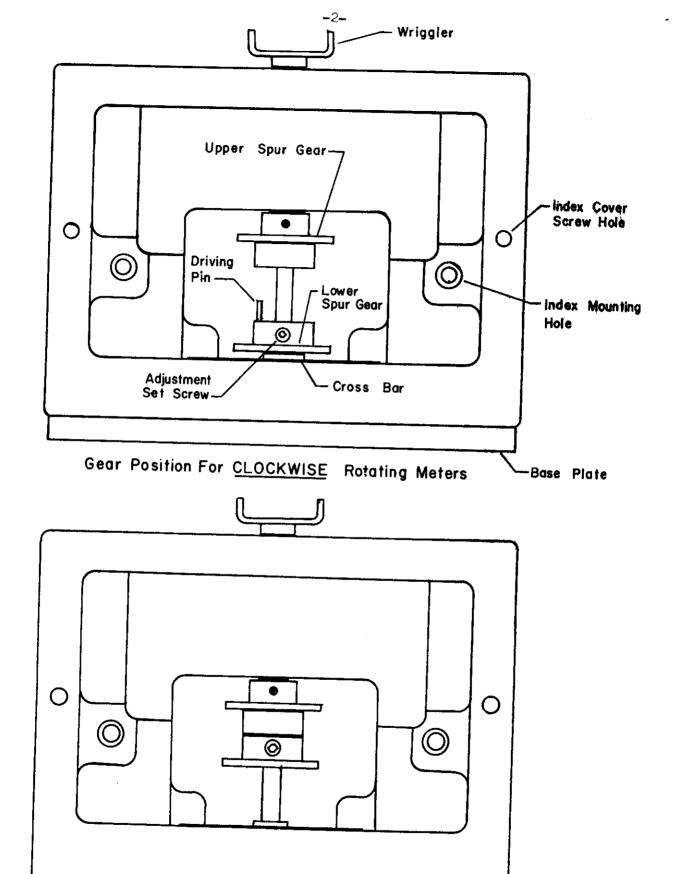
Gear Position For COUNTER-CLOCKWISE Rotating Meters
