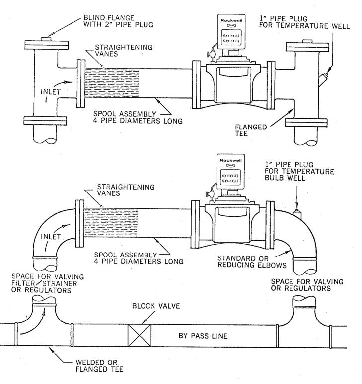
NOTE: Straightening vanes are required on short-coupled Turbo-Meter sets for maximum measurement accuracy
