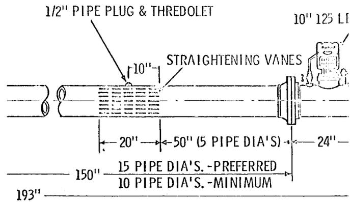
NOTE: NO SPECIAL SUPPORTS REQUIRED TO HOLD METER, STANDARD PIPE ARE SUFFICIENT.
