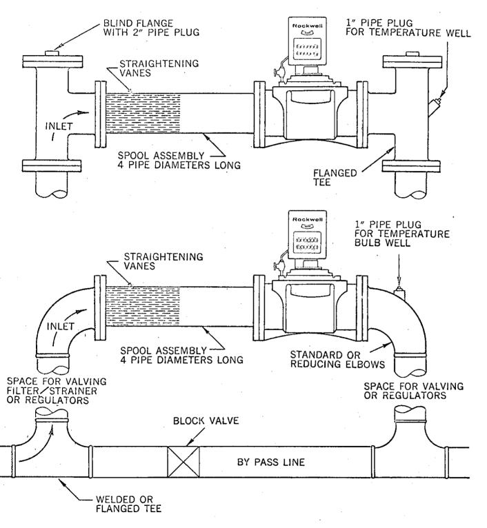
NOTE: Straightening vanes are required on short-coupled Turbo-Meter sets for maximum measurement accuracy
