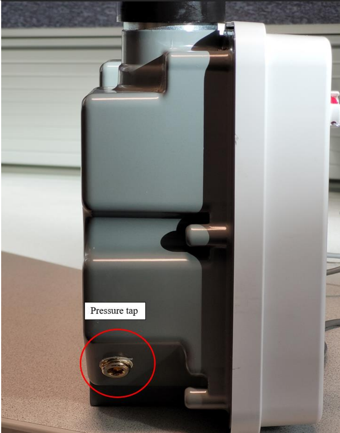
Figure 2: Sonix IQ location of the pressure tap / Sonix IQ emplacement de la prise de pression
