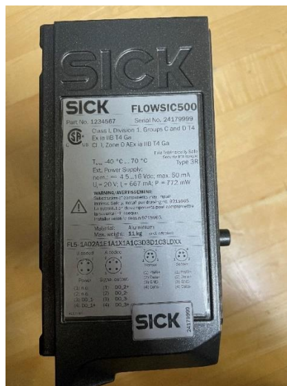
Figure 7 - Additional seal on nameplate / Scellage additionnel sur la plaque signalétique
