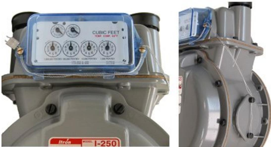
**Figure 2.** Sealing provisions / Dispositifs de Scellage
