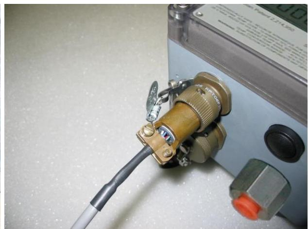
**Figure 7:** Wire seal on AdEM-PTZ electronic compartment and output pulse connector as well as wire integral seal / Fil métallique et scellé sur le compartiment électrique et sortie d'impulsion du AdEM-PTZ
