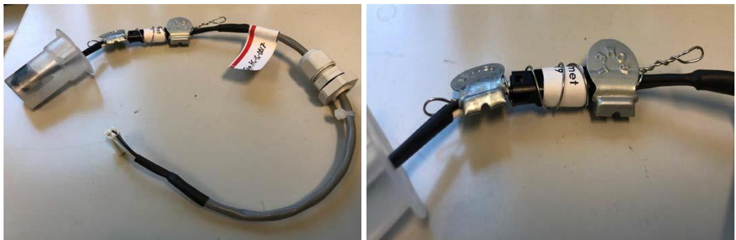
**Figure 17:** Typical sealing of the interchangeable Wiegand sensor assembly / Scellage typique de
