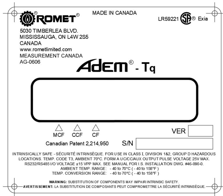
**Figure 13:** AdEM-Tq nameplate – used for imperial and metric configuration.
