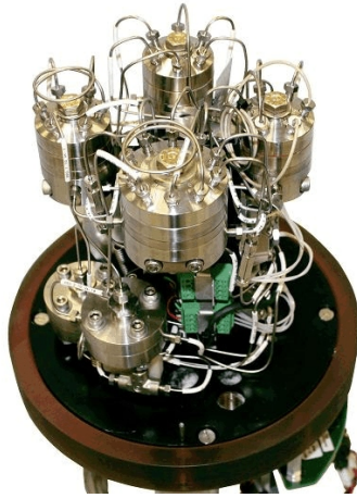
Figure #2 / Figure n° 2 Oven Assembly / Four
