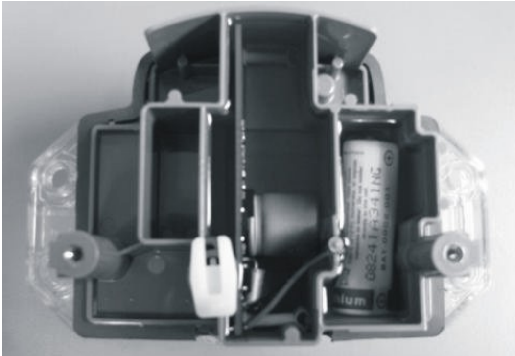
Figure 13: 100G Datalogging ERT, Part No. ERG-5002-001 (Front View) / No de pièce ERG-5002-001 (Vue de face)
