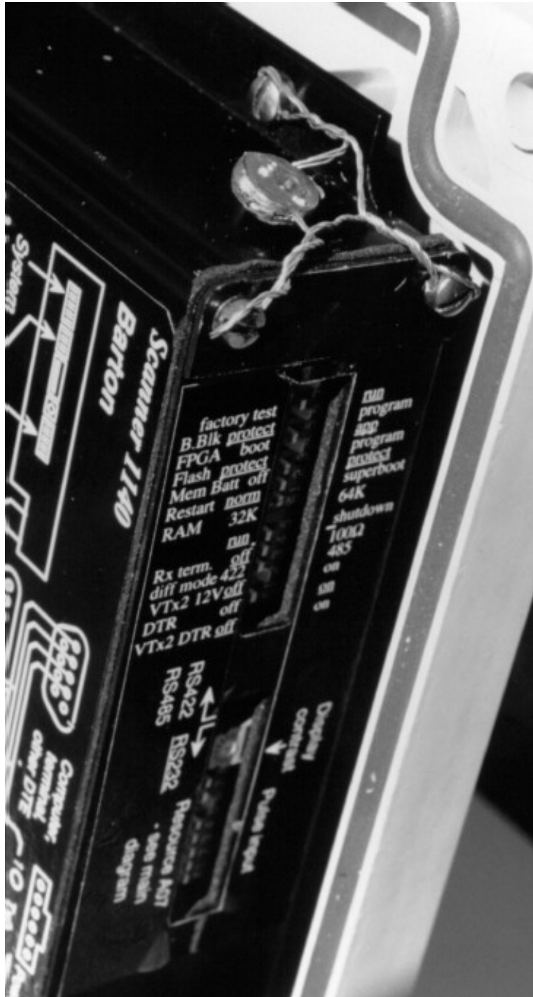
Figure 6 : Sealing Provision / Disposition de scellage
