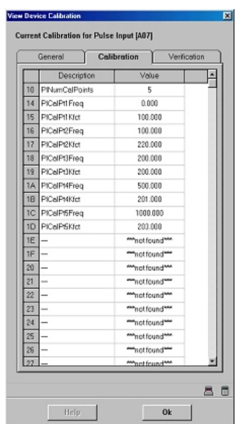
**Figure 4** Device calibration window/Fenêtre Device calibration
