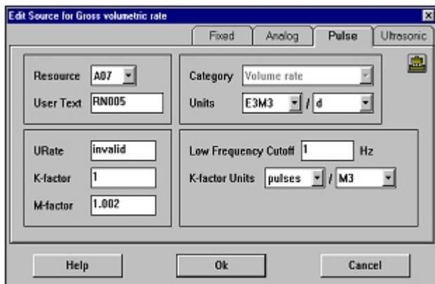
**Figure 3** Edit source window/Fenêtre Edit Source
