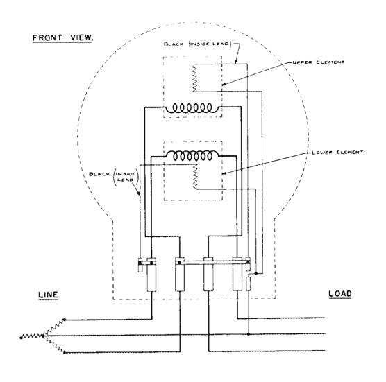
INTERNAL & EXTERNAL WIRING FOR TYPE
