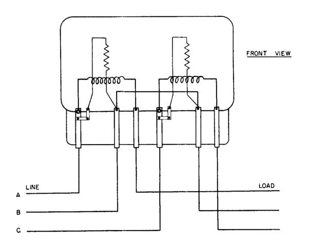
CONNECTION DIAGRAM FOR S3 HORIZONTAL POLY. METER. 6 TERMINAL SELF-CONTAINED ON 3 PHASE, 3 WIRE SERVICE
