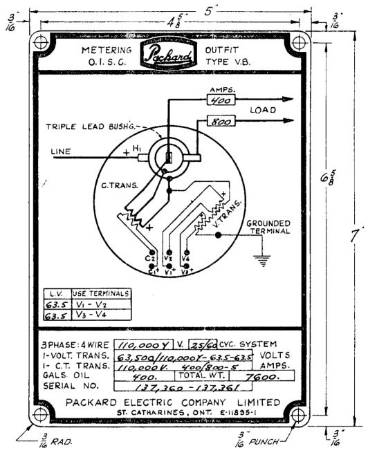
PLATE ETCHED ON .025 STAINLESS STEEL,
