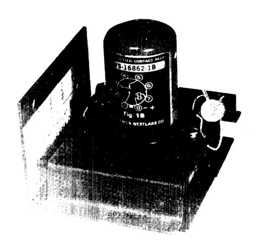
The metal terminal cover has a hole in the centre through which the octal relay socket protrudes. A metal ring with drilled tabs slips down over the flange at the base of the relay. The relay and terminal cover are both sealed by passing sealing wire through the drilled tabs and matching holes in the cover. The terminal cover screws are rendered inaccessible by the ring. For outdoor use this device must be mounted in a weatherproof enclosure.
