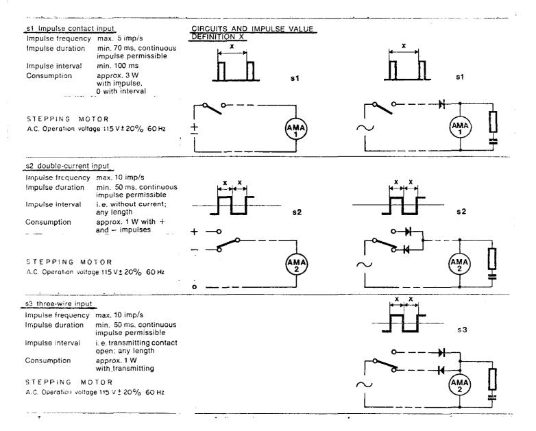
NOTE: The broken lines indicate transmission lines.
