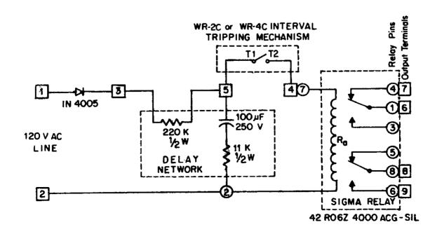
Canadian Westinghouse types WR-2C and WR-4C Demand Recorders have received approval when factory equipped to serve as a "Master" recorder. This entails the addition of a dry reed switch and appropriate wiring to case terminals "Tl" and "T2".
