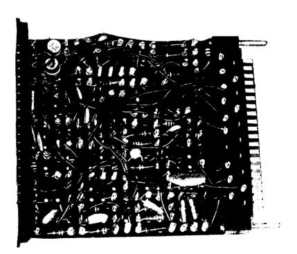
The type SST-1 Totalizers are of modular construction with each module in a separate dust-proof housing. The modules are socket-mounted on the chassis and interwired as required for the particular system. The pulse counters are mounted on a separate panel for semi-flush mounting on the switchboard face. The module chassis are designed for mounting on a 19 inch relay rack or on the back of a switchboard. Each module has an identification number painted on the top which describes its function.
