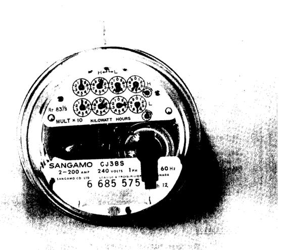
Each register has its own test dial and the multiplier of 10 applies to both registers.
