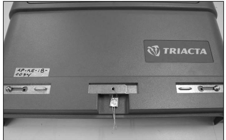
**Utility seal used with exposed terminal card /
