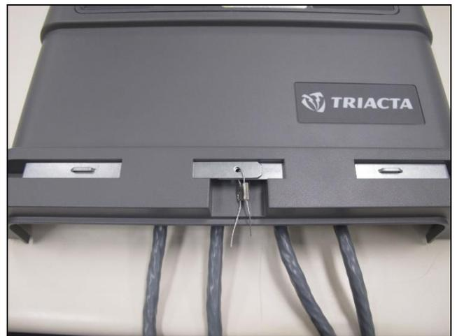
**Utility seal used with overmolded terminal card /
