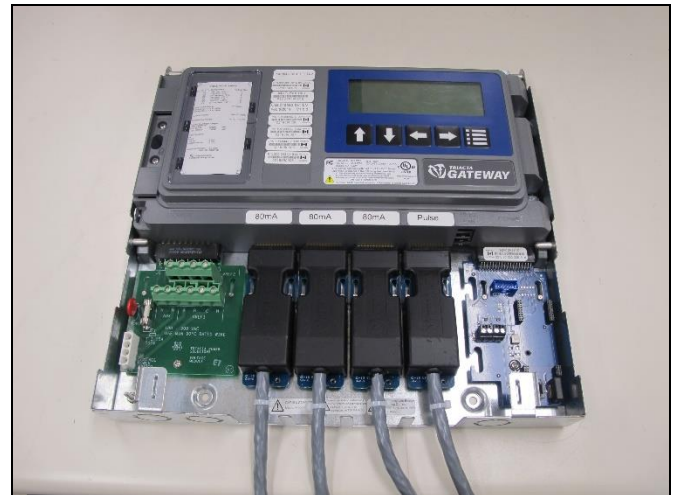
Overmolded Terminal Cards / Carte bornes moulée
