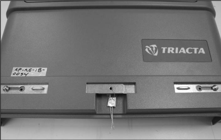
**Utility seal used with exposed terminal card /
