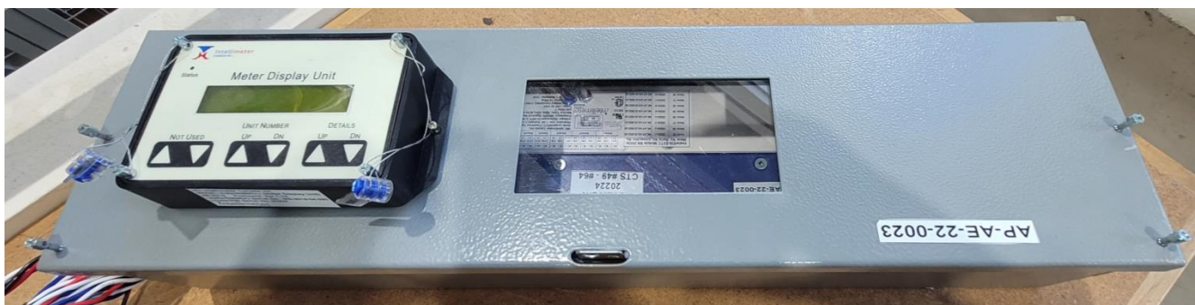
i-meter636-EXTC Meter with new enclosure, single module version. / Compteur i-meter636-EXTC
