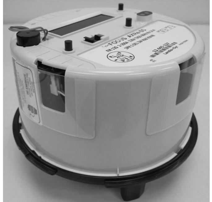
**Polycarbonate shields placed over the meter housing
