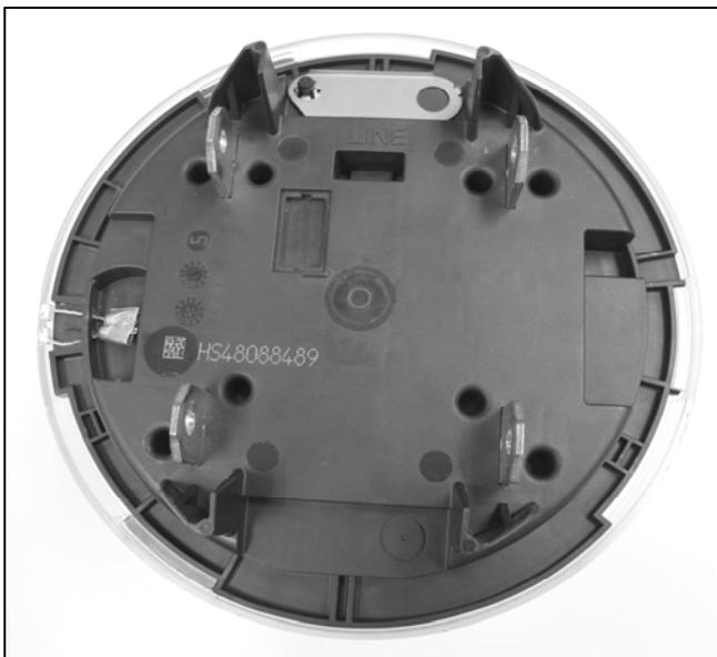
**Sealed CENTRON II C12.19 with molded test link plug
