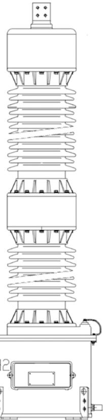
**arteche** CAPACITOR VOLTAGE TRANSFORMER
