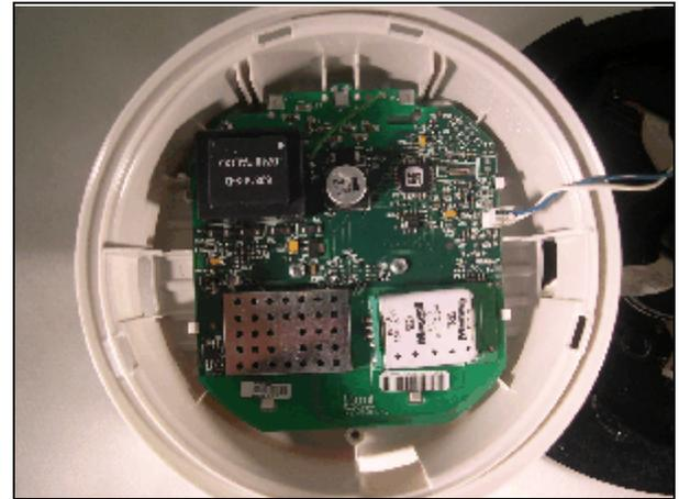
**Board with Integrated StatSignal
