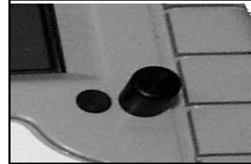
Sealing Plug - Fitted / Bouchon de scellage - inséré
