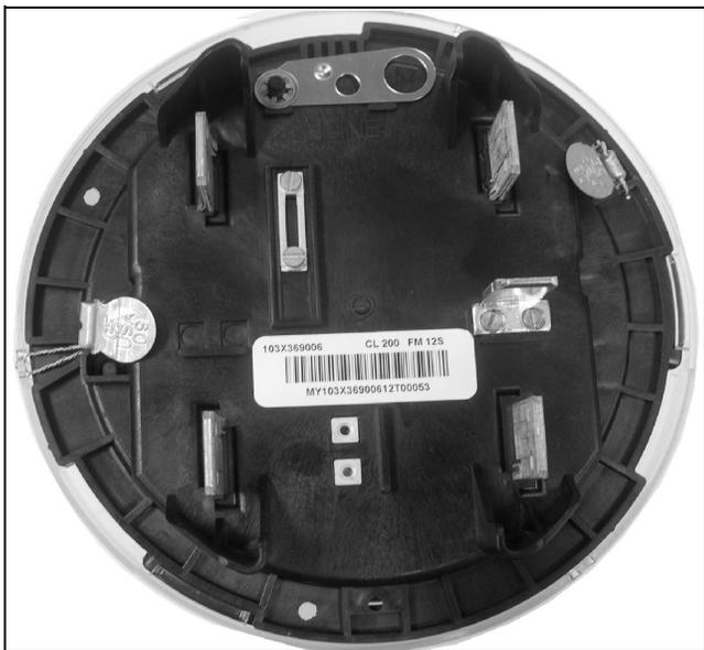
**Rev. 6 New sealing method: two seal/barrier**
