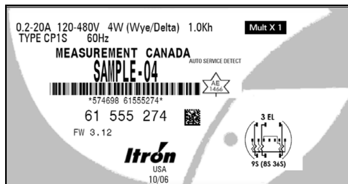
Centron CP1S Nameplate / Plaque signalétique Centron CP1S
