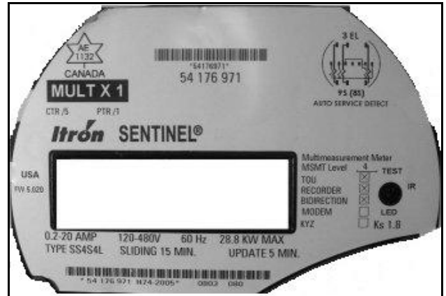
Rev. 11 Sentinel with Trilliant Networks NCZR801PH-Sent SecureMesh™ module nameplate / Rév. 11 Plaque de Sentinel avec module NCZR801PH-Sent SecureMesh™ de Trilliant Networks
