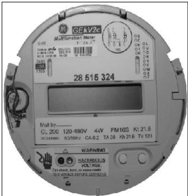
KV2c retrofitted with 53ESS Itron module/
