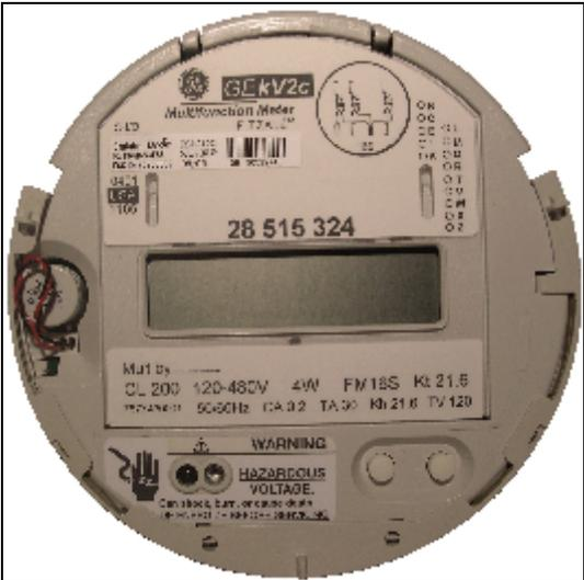
KV2c retrofitted with 53ESS Itron module/
