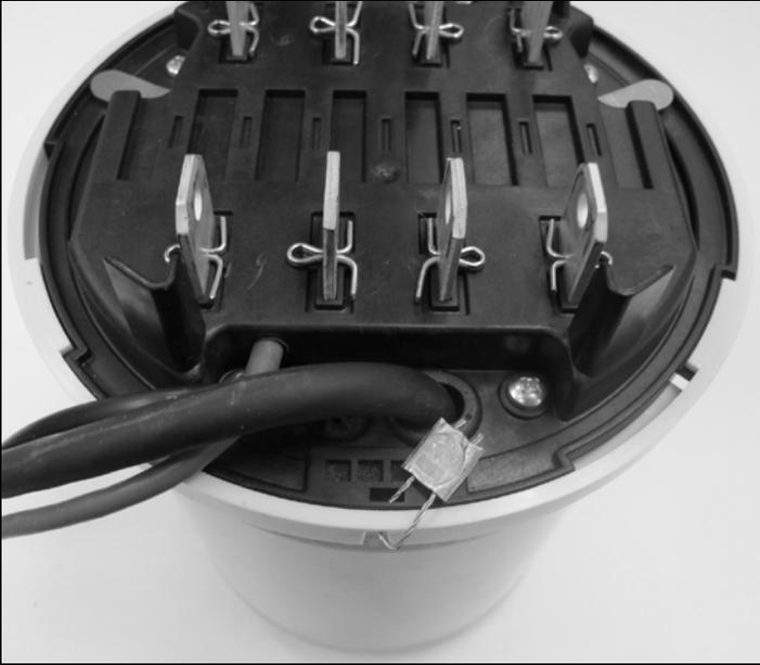
Sealing of the JEMStar meter prior to revision 4 /
